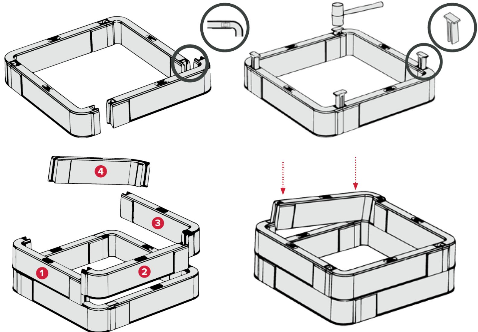
Step 1 – Arrange parts to match opening dimensions – See color coded drawing of chamber.
