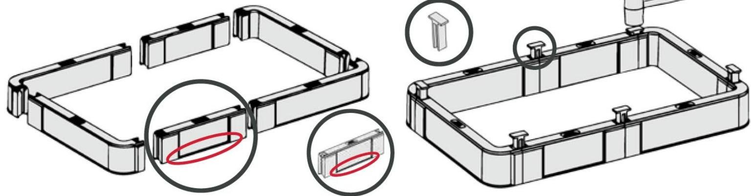
Step 2 – Alternate right and left parts as you add sections to the chamber, this provides “brick works” and is crucial for stability and strength. Straight parts can be used in all sections of the chamber.
