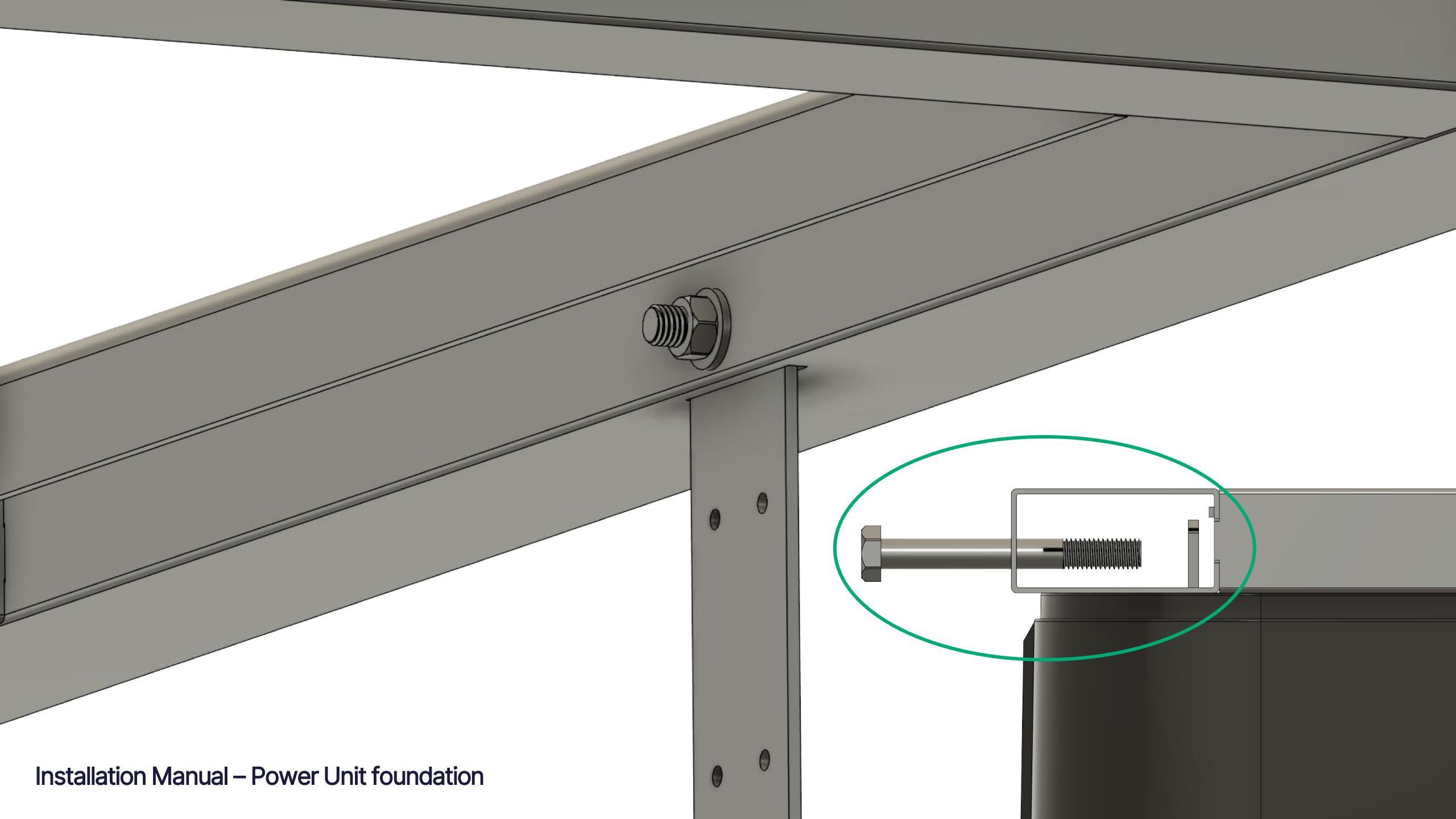
→ Step 3: Use self-tapping screws to secure steel frame to foundation
