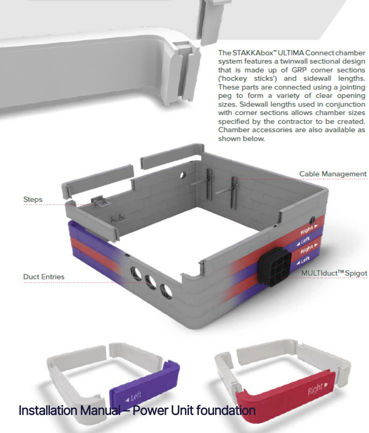
The STAKKAbox™ ULTIMA Connect chamber system features a twinwall sectional design that is made up of GRP corner sections ('hockey sticks') and sidewall lengths. These parts are connected using a jointing peg to form a variety of clear opening sizes. Sidewall lengths used in conjunction with corner sections allows chamber sizes specified by the contractor to be created. Chamber accessories are also available as shown below.
