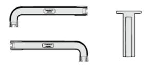
a) Arrange corner sections to match the chamber clear opening dimensions. The corner sections should be all 'left' or all 'right' on each section and will alternate between the two as the chamber increases in depth. b) Connect the sections using jointing pegs, ensuring that the top of the peg is level with the top of the section. All pegs should be partially inserted before tapping home.
