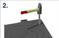
Using the punch supplied, tap out the veneer of iron in the knock out well in the primary cover section
