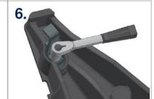
Fully tighten with a 22mm socket or similar tool, taking care not to overtighten. \*
